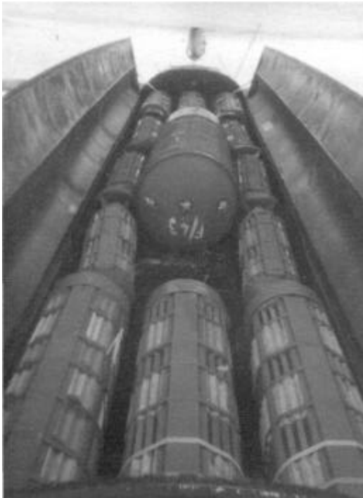
An enormous array of incendiaries surround the “cookie” in this cavernous Lanc. bomb bay
