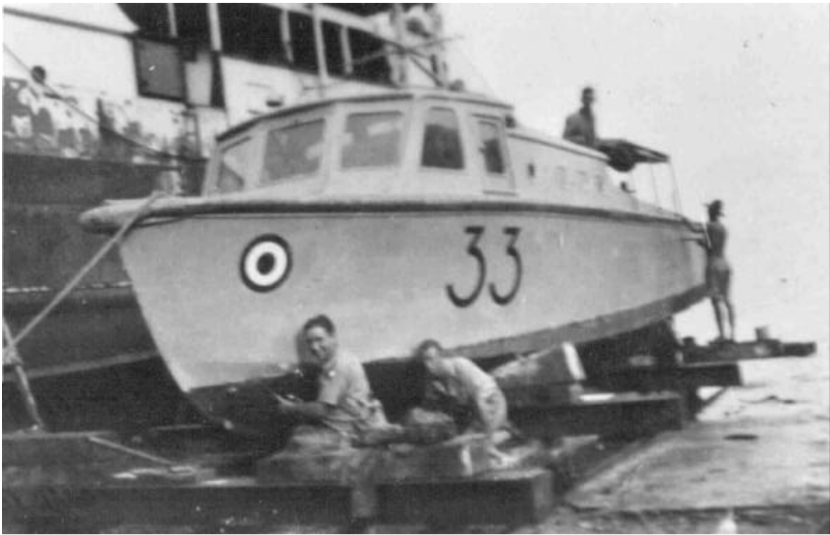
A Marine Section Boat on the slipway in Port Moresby, 12.10.42. Claude Shaw, Col Fountain and Jack Angula were hard at work completing the antifouling. (Cliff Searle)
