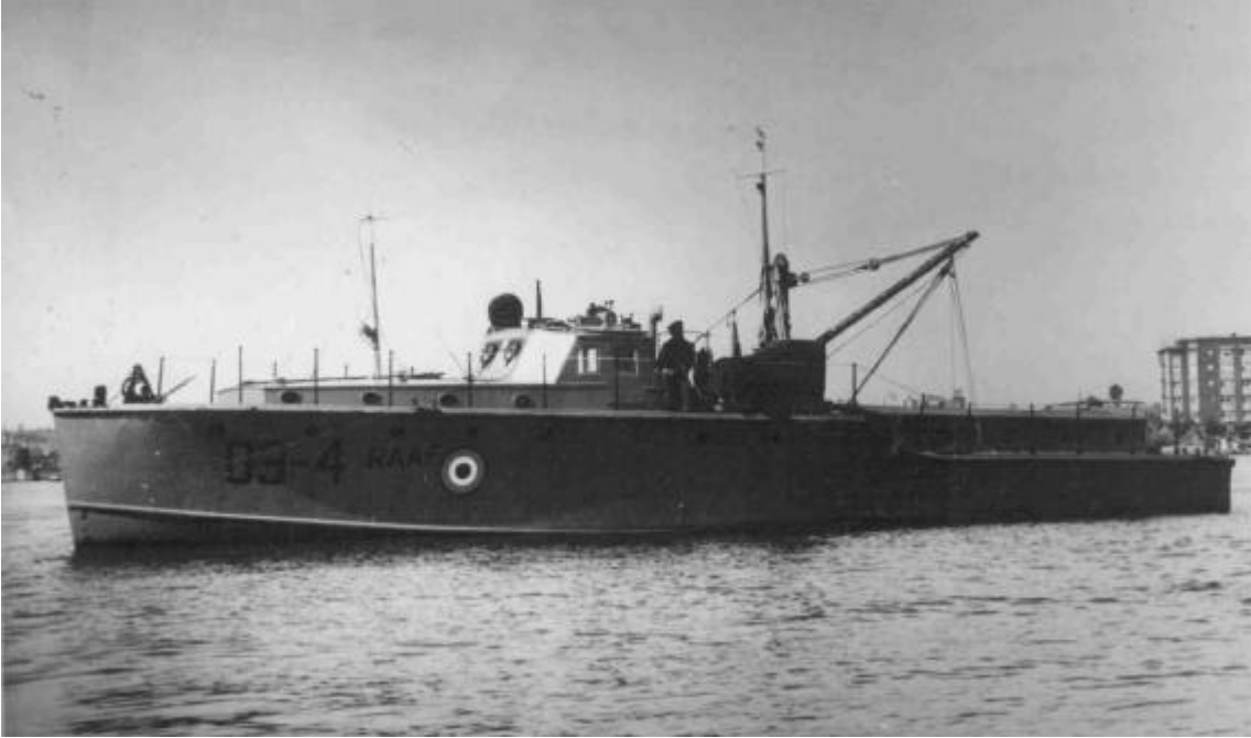
The heavy duty lifting hoist of a Torpedo Recovery Boat can be more clearly seen on 03.4 (Alf Wilson)
