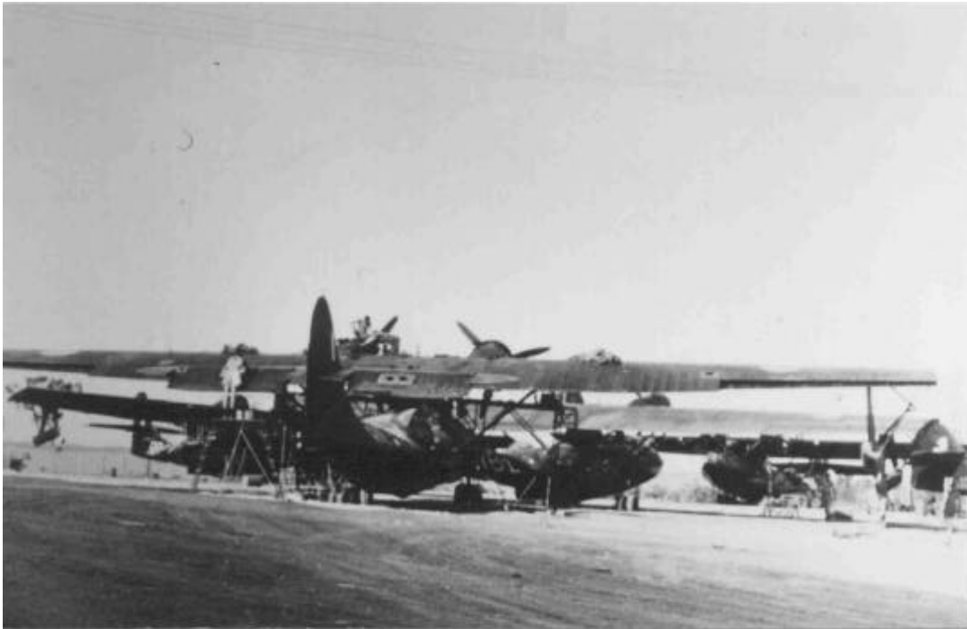
At RAAF Base East Arm Catalinas were fitted with wheels so that they could be hauled up the slipway then onto the hard for servicing. Only a few RAAF Catalinas were amphibians. (Doug Hamilton)
