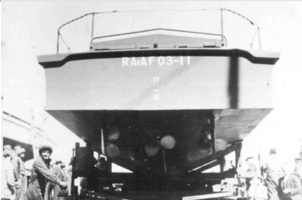
03.11, newly built by Harold Chandler, will soon be in the hands of the Marine Section. Three propellers can be clearly seen. (Kitch Williams)
