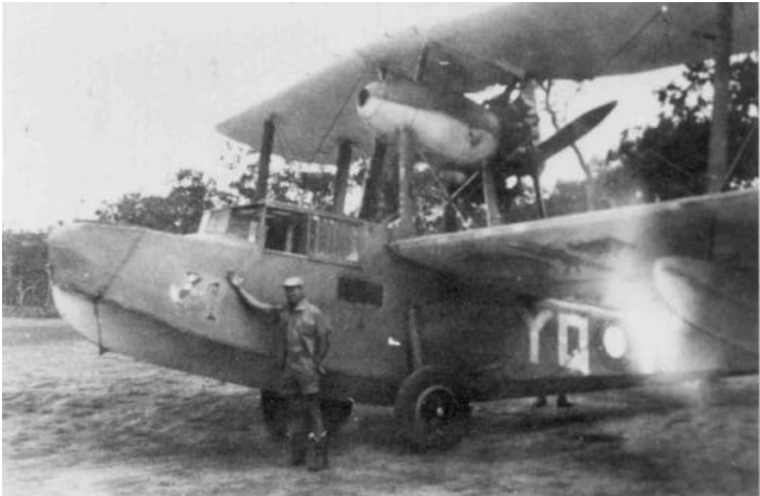
Originally these aircraft were known as Seagull Mk. 5 and flown by RAAF Pilots from RAN (Navy) Cruisers. When the RAF had them built they called them "Walrus". but their wings were not hinged. (Frank O'Brien)
